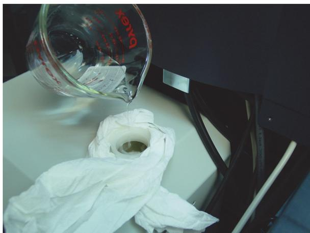
Figure 10.5 Adding coolant to the ThermoCube unit
