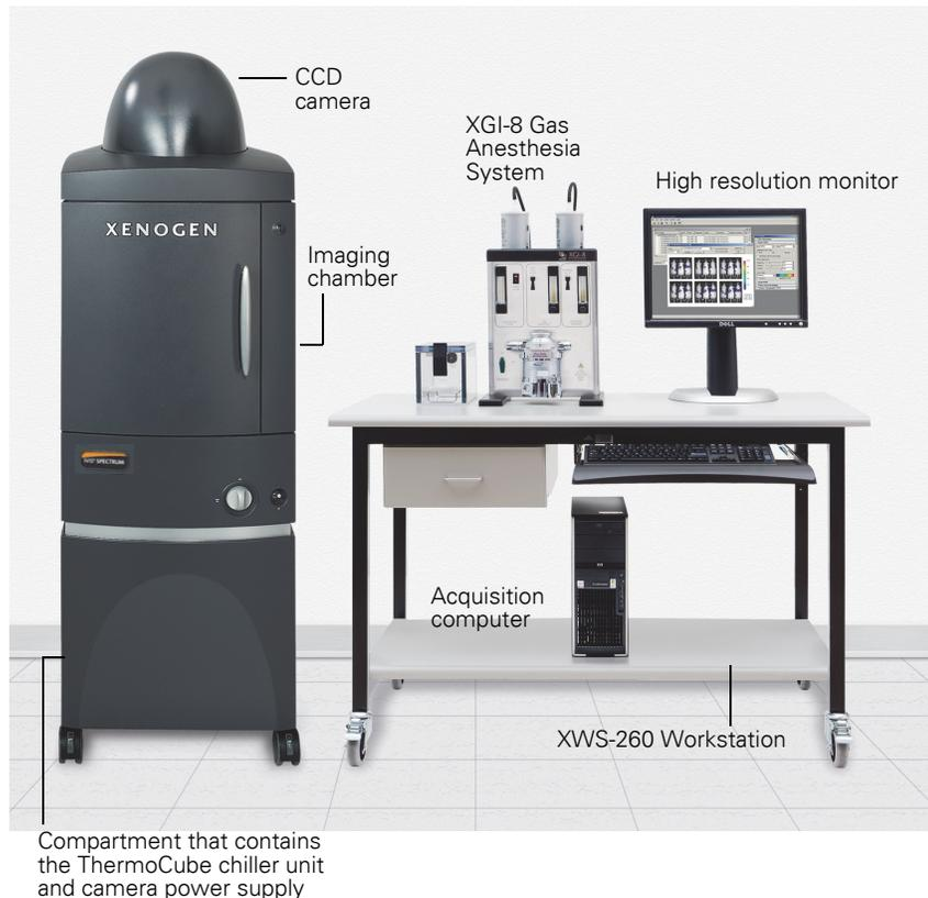
**Figure 1.1** IVIS® Spectrum Imaging System
