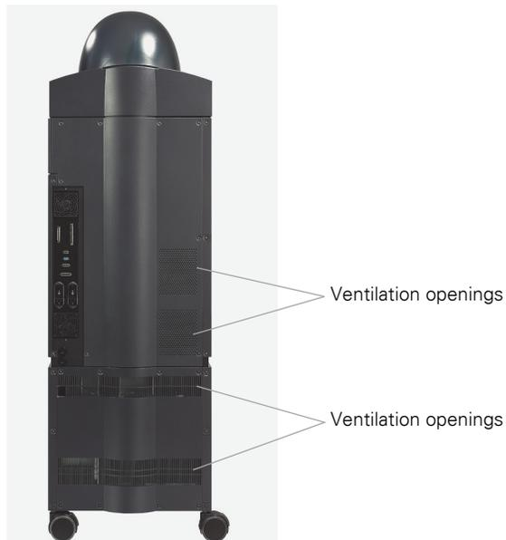
**Figure 6.7** IVIS Spectrum, back view
