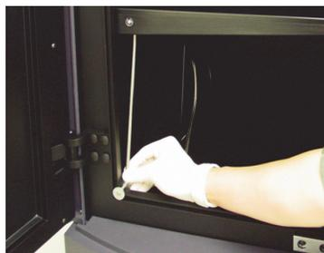
Pull the bar down from the stowed position and place it as shown above. Return the bar to its stow position before returning the imaging platform to the operating position.
